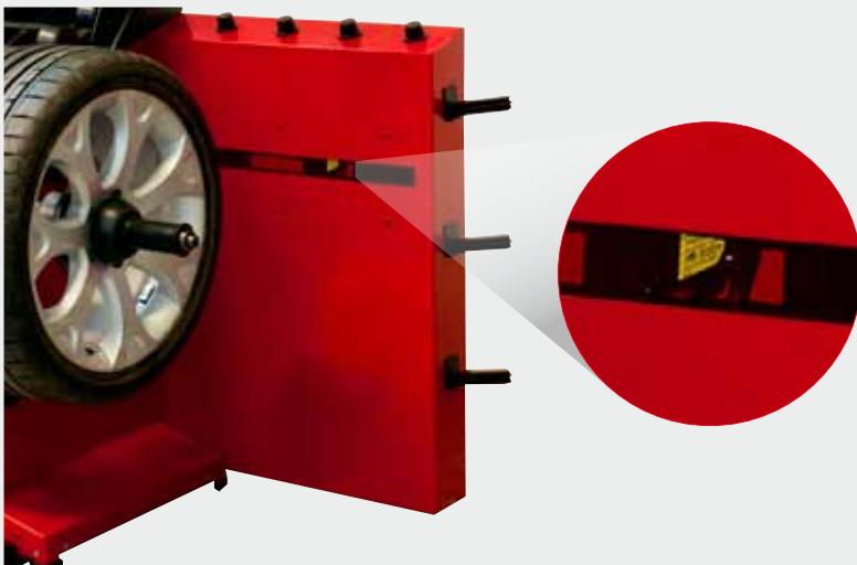
High precision laser sensors automatically measure **all wheel dimensions** in a few seconds during the measurement cycle.
