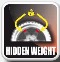
Keeps rims looking great by dividing the external side balancing adhesive weight into two equivalent weights applied in hidden locations behind the spokes.
