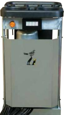
The **electro-hydraulic power unit** with display can be positioned as desired and allows the user to **save all the data** relating to the tyre being processed.
