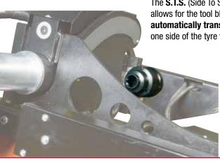
The **S.T.S.** (Side To Side) device allows for the tool block to be automatically transferred from one side of the tyre to the other
