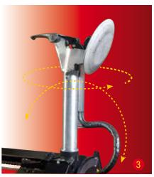
Bead breaker disc sequence of automatic movements:
