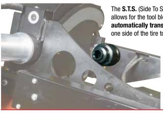
The **S.T.S.** (Side To Side) device allows for the tool block to be automatically transferred from one side of the tire to the other
