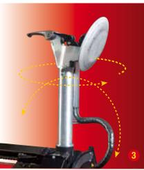
Bead breaker disc sequence of automatic movements:
