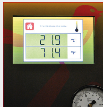
20-25°C, green = work on tire may proceed normally
