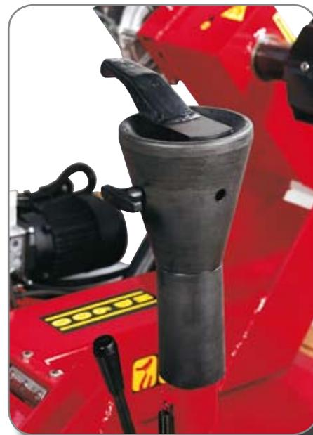
Special tool for tube-type and supersingle wheels
